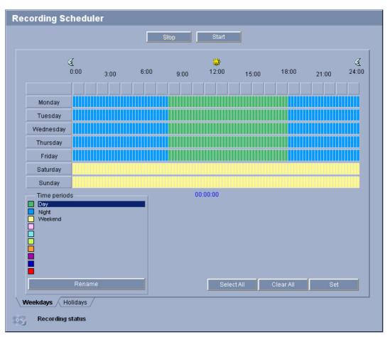
The recording scheduler allows you to link the created recording profiles with the days and times at which the camera's images are to be recorded in the event of an alarm.
